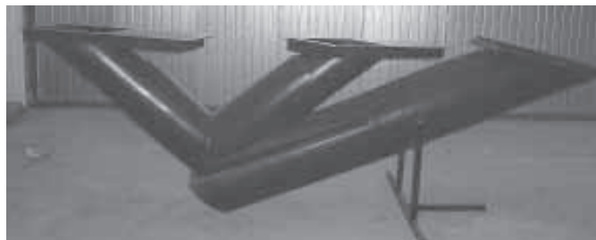
This set of angled 12-in. dia. poly pipes is buried under bin, eliminating the need for hopper bottoms or unloading augers.
