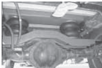
TLC kit adds the benefit of coil and air springs to the original leaf springs, says the company. It fits all Ford, Chevy and Dodge 1/2-ton trucks.
