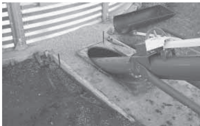
To unload a bin, you slide an auger into the outer opening and open one of the slides inside the bin to get the grain flowing.
