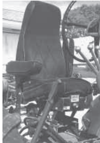
There's no air compressor. Beck uses a shop compressor to fill the seat's airbag.
