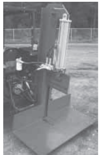
Operator uses a control lever on the tractor to raise and lower the platform, and another lever on the splitter to operate the cylinder, which has a cycle time of about 8 seconds.
