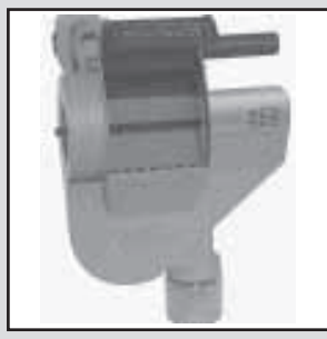
Hand-held unit threshes the grain and deposits it in a glass jar for moisture testing.
