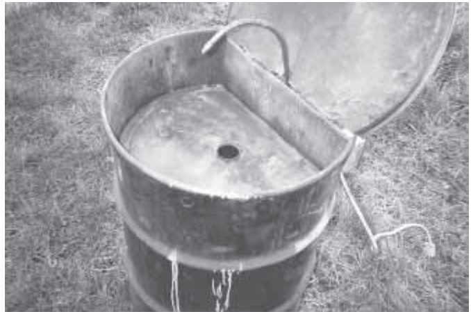
Lowe made his own parts washer out of a 55-gal. barrel and an electric, recirculating submersible solvent pump. Note removable wash tray 8 in. down from barrel's lip.
