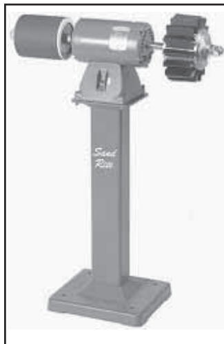
Contour sander features both a pneumatic sanding drum and a unique brush-type sanding head.
