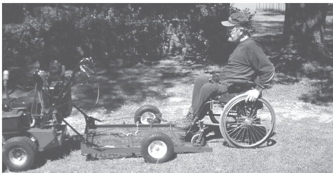
Trailer's bed is raised and lowered by means of a cantilever system that's connected to both wheels. Hinged tailgate on back of trailer also raises up.
