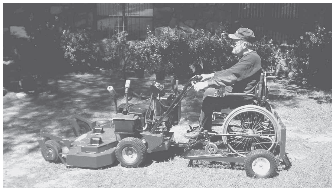
Home-built 2-wheeled trailer lets Don Bragdon operate his Snapper walk-behind mower, equipped with a 48-in. deck, right from his wheelchair.
