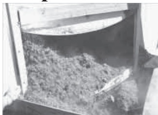
Compost can be discharged from the in-vessel composter after just three days.
