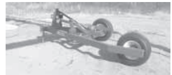
Caddy has an adjustable top link and an adjustable front hitch for leveling the mower.
