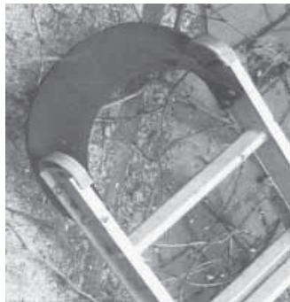
Twisted tire sidewall provides slip resistance against buildings. It also flexes to center the ladder on objects that aren't flat.
