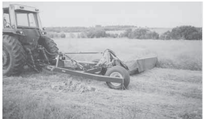
Caddy makes it easier to hook up to a 3-pt. mounted disc mower and also reduces the amount of power required to pull it, says the manufacturer.
