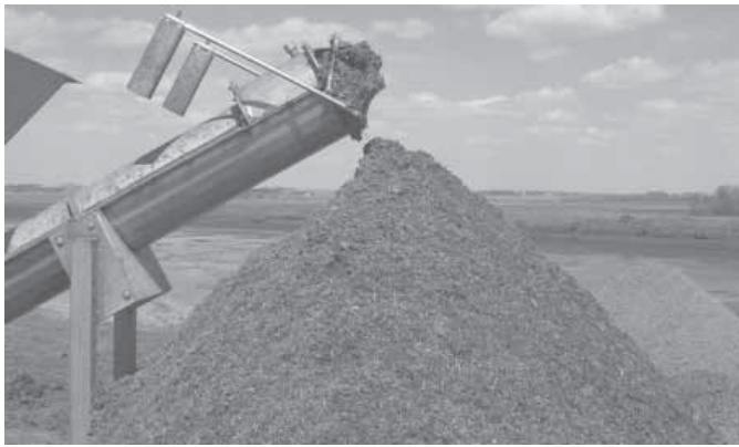
“Manure Monster” dewatering system separates liquids from solids.
