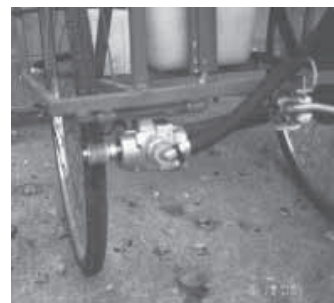
One of the bicycle wheels friction-drives a 1 1/2-in. dia. wheel that powers the pump.
