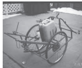
Sprayer rides on a pair of 26-in. high bicycle wheels and is equipped with a 5-gal. poly tank and 4-roller HyPro pump.
