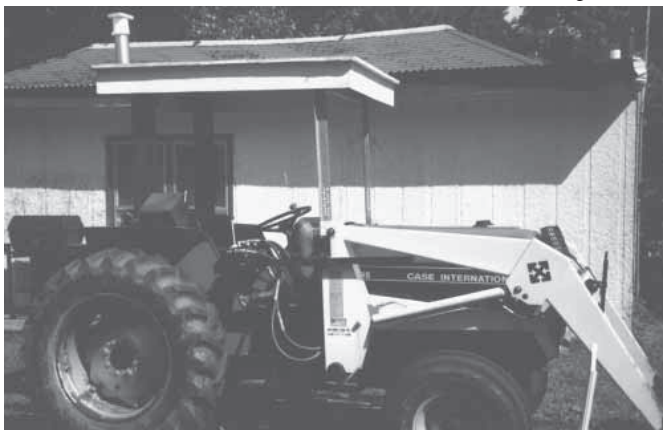
Canopy’s roof is made from plywood covered by sheet metal.
