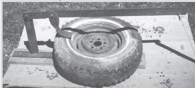
A 2 1/2-in. long upright has several holes drilled in it to adapt to different size tires. A 60-in. pry handle pins to the upright, and a curved bead-breaking shank hangs down from under it.
