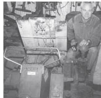
Bob Bugger added an oil bath air cleaner off an old late 1940's Massey Harris tractor to one side of his White riding mower.
