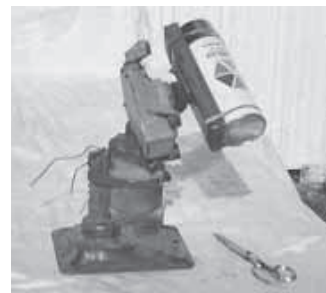
Automatic “revolver” rotates the can around and around to thoroughly mix paint.
