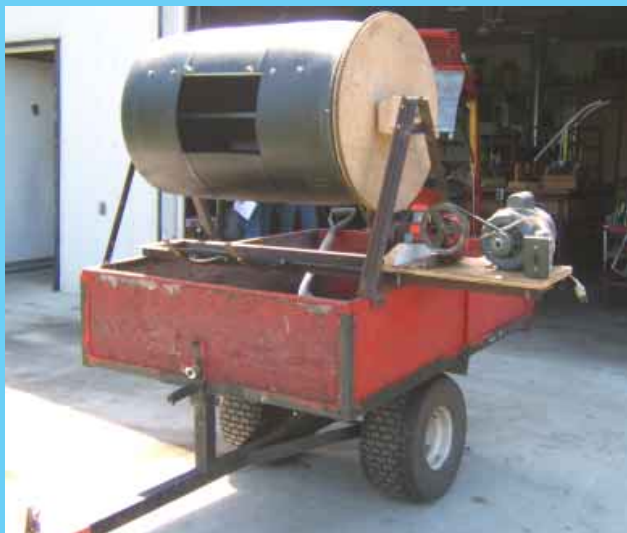
Soil mixer consists of an old 45-gal. plastic antifreeze drum that serves as the mixing chamber. Barrel is rotated by a 3/4 hp electric motor.
