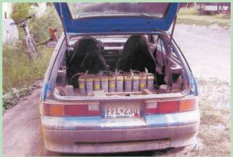
Kilian Herrington converted this 1991 Geo Metro with an electric DC motor for daily use. The motor is powered by nine 12-volt batteries carried in the back.
