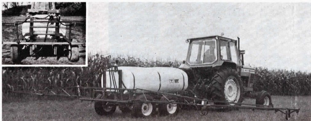
Linkage design of self-leveling boom (see inset photo) keeps boom parallel to ground, even on slopes and sidehills.
