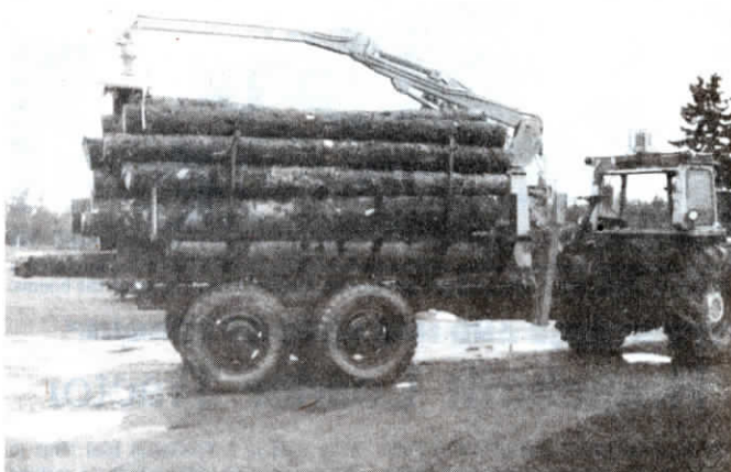
Burns installed the lift arm on a wood-hauling trailer he built out of an old army truck.
