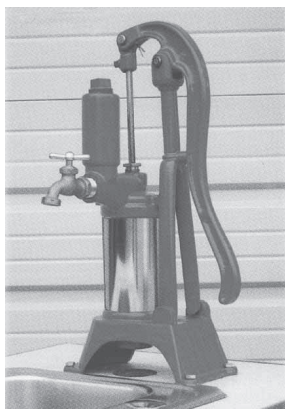
Jim Smith installs old hand pumps that draw from springs, rainwater cisterns and even deep wells.
