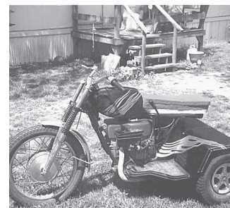
To build mini chopper, Jennings connected an old Honda motorcycle frame to the rear end off a Murray garden tractor.
