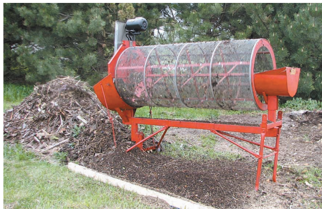
Black turned a rotary grain cleaner into a compost sifter, replacing the screen with hardware cloth.
