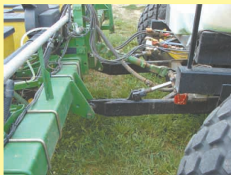
Mike Peterson fashioned the rugged 3-pt. hitch on back of the fertilizer cart. Two cylinders raise and lower the bar.
