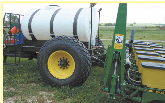
Homemade and handy, this 2-wheeled cart carries 1,000 gal. of liquid fertilizer while carrying an 8-row planter on a 3-pt. hitch.
