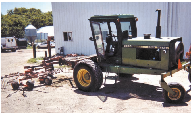
Self-propelled twin tandem Kuhn rake was built out of a Deere 3830 swather.
