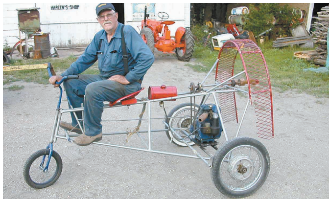
Harlen Grovom's "air cycle" gets a lot of chuckles at parades. The rider is pushed along by a 30-in. propeller belt-driven by a 7 hp Wisconsin air-cooled engine.
