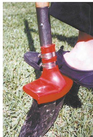
Molded plastic attachment fits over top edge of shovel. It has a 3 1/4-in. wide lip, so you step down on a much bigger area.
