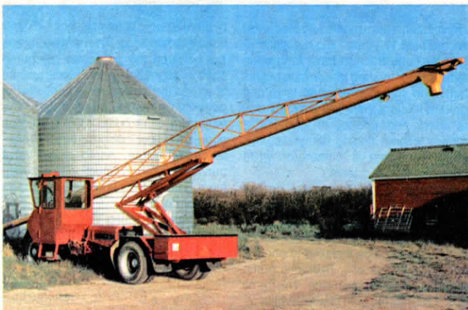
To unload bins, the input end of the auger can be driven up to the bin door to work its way inside.
