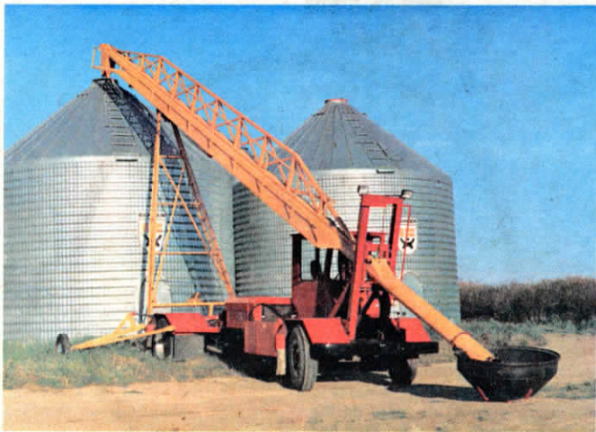
Newest 10 in. by 60 ft. auger shown with stabilizers fully extended to 18 ft.
