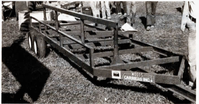
Wood's header carrier, loaded with an 8 row head, and sitting empty, below. Heads are simply set onto trailer with the combine, then towed down the road on the trailer.
