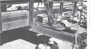
A 12-volt winch is used to chain-drive trailer's tongue jack. Shaft that runs to side of trailer can be cranked by hand if power fails.
