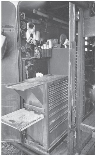
Toolbox is on one side of trailer and has a pair of hinged fold-out working tables on it.
