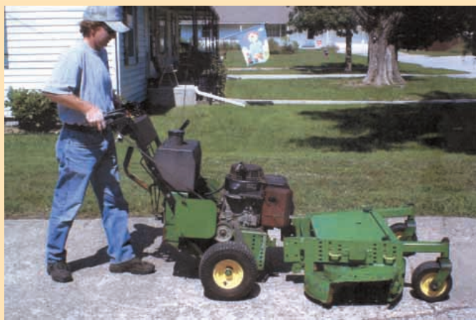
Kevin Gliser converted this Deere walk-behind mower into a power unit that's designed to quick-tach to a variety of implements.
