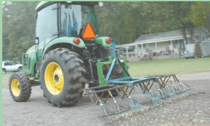
"People laugh at it until they see the results," says Bartt Nettleman about his 3-pt. mounted raking contraption. He uses it to clear leaves off a 20-acre campground.
