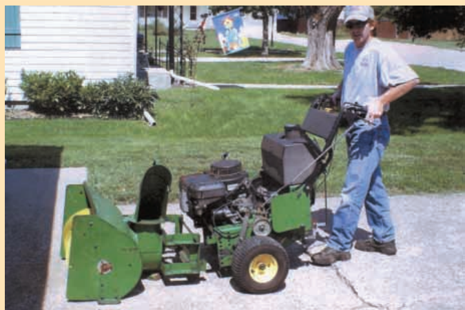
The original belt-driven power system was converted to pto drive, and he added quick-tach brackets that let him switch attachments without using tools.
