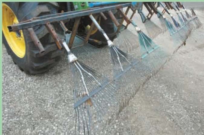
He welded up a 9-ft. wide frame out of 1-in. tube steel with pegs to hold two rows of steel broom rake heads.
