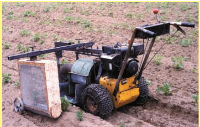
He guides the snowblower between two rows, with the screened cage located on the opposite side of the row just brushing the leaves.
