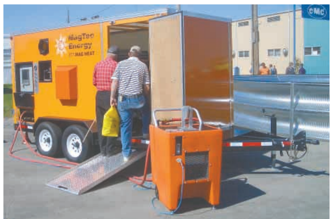
Magnetic heat system is housed in trailer. Portable heat unit, hooked to cables, can be used up to 400 ft. away.
