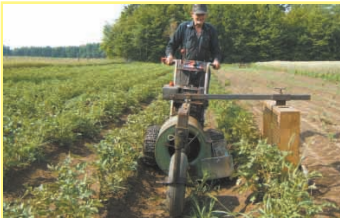
Eric Campbell gets rid of potato bugs by using a furnace fan - mounted on a 10 hp snowblower - to blow them into a screened wooden cage.
