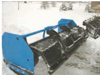
Snow plow collar pops on and off a snowplow, turning it into a snow pusher box.
