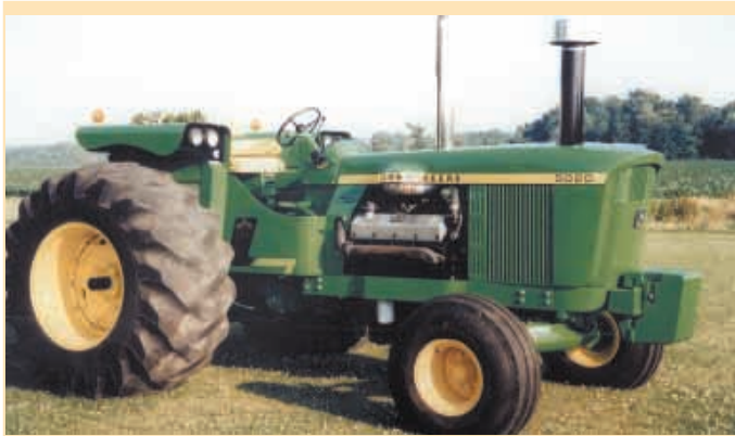
"It looks nice, almost like it was installed by the factory," says David Agle of Collins, N.Y., who repowered his Deere 5020 with a used Cummins V-8 turbocharged diesel.
