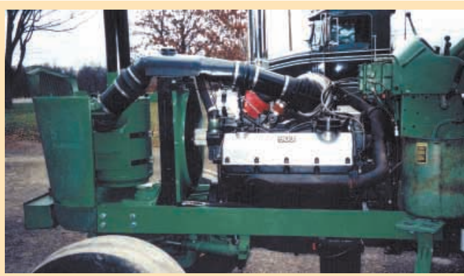
A metal pipe with a sharp elbow in it leads from the air cleaner, over the top of the radiator to the intake side of the turbocharger.
