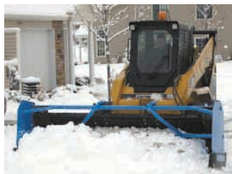
Snow plow collar pops on and off a snowplow, turning it into a snow pusher box.
