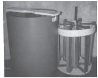
"Radial" honey extractor was built using the brine tank from an old water softener.
