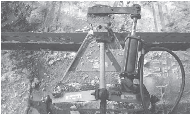
Kramer added 1 ft. to each side of his 7-ft., 3-pt. mounted blade. Add-on hydraulic cylinder lets him easily adjust direction from tractor seat.
