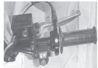
A cable runs from foot throttle up to ATV handlebars to control twist grip throttle.
