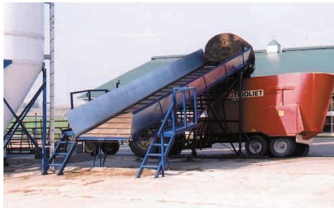
Bales are moved up the elevator by 5-ft. wide manure spreader floor chain.
