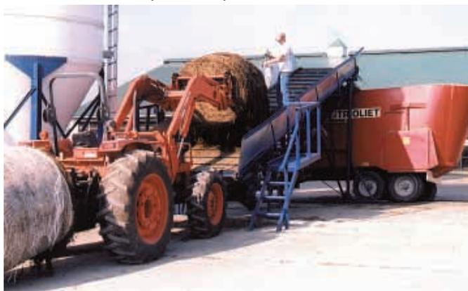
Home-built 30-ft. long, 12-ft. high elevator is used to load silage bales into Clavin’s tub grinder.
