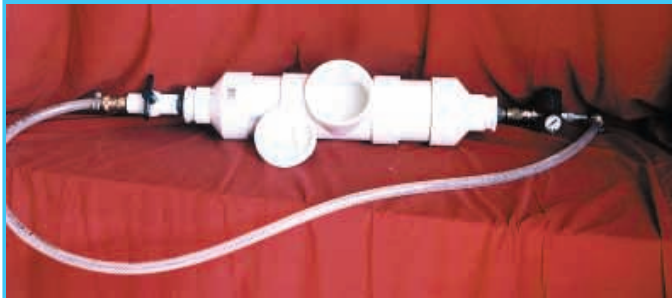
Injector is made from a 4-in. pvc cleanout tee with a threaded plug in the tee.
