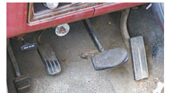
A second gas pedal installed on the floorboard controls wood gas flow.
