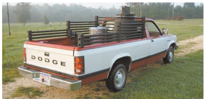
Wayne Keith uses scrap wood, left over from his sawmill business, to power his 1987 Dodge pickup.
