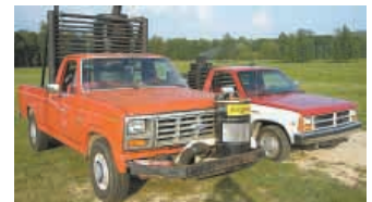
A 30-gal. barrel on a platform over the front bumper is filled with hay and serves as a filter for cooled gases.
