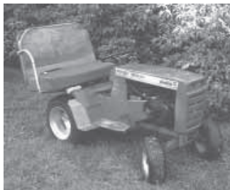
Burg mounted a school bus seat on back of his Wheelhorse 12 hp garden tractor.
