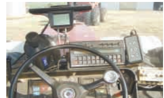
The boom (above) was built in three sections and rides on a pair of big gauge wheels which help it float over uneven ground. Tractor cab is fitted with an E-Z Steer automatic guidance system. They made special mounting brackets to mount it to the cab's frame.
