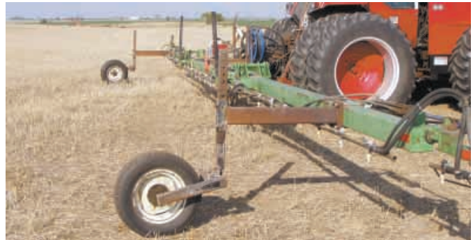
The boom (above) was built in three sections and rides on a pair of big gauge wheels which help it float over uneven ground. Tractor cab is fitted with an E-Z Steer automatic guidance system. They made special mounting brackets to mount it to the cab's frame.
