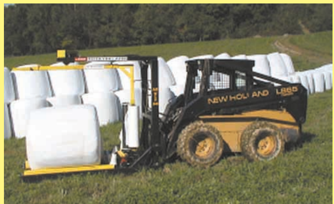
Universal quick-tach adapter plate allows bale wrapper to be quickly mounted on any brand of skid steer loader using just three pins.
