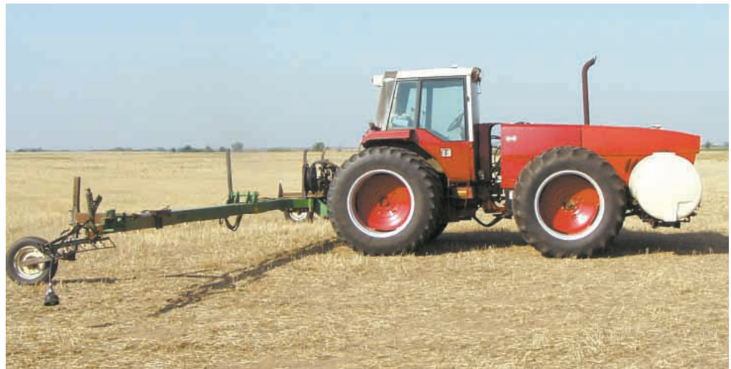
"It has many of the same high-tech features found on expensive self-propelled sprayers, yet cost less than $16,000 to build," say Leon Becker and Norbert Meyer about their home-built, 3-pt. mounted sprayer. It's mounted on an IH 3588 articulated, 4-WD tractor.
