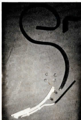
New applicator shank combines the strength of a springtooth shank with the light draft of a coil shank.
