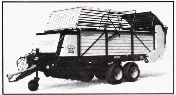
New chopper wagon dumps its load out the back or feeds it into bunks with a side-unload conveyor. All moving parts are openly accessible for maintenance and service.
