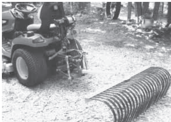
Home-built electric lift hitch is equipped with a 2-in. receiver hitch and is powered by a winch that operates off the tractor's battery. Inventor Stephen Ferrante uses it to pull a 4-ft. wide rake that he built himself.
