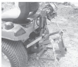
Winch mounts on top of a vertical metal channel that's attached to a pair of hinged metal frames.
