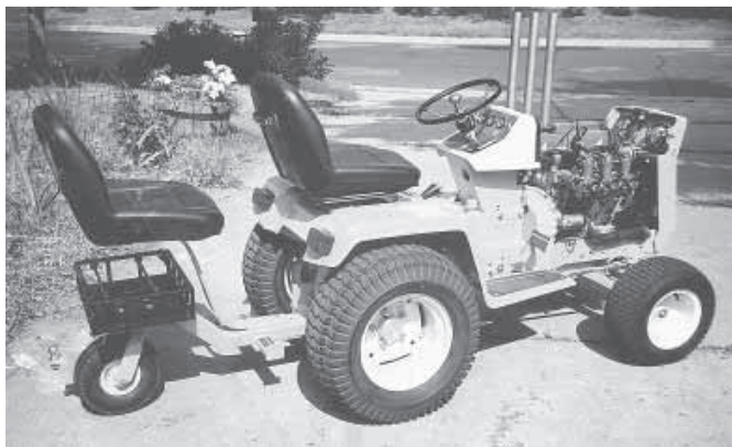
Just for fun, Carlo Shefveland and Dale Lemmerman repowered this 1970 Cub Cadet garden tractor with a Geo Metro 3-cyl., 60 hp car engine.
