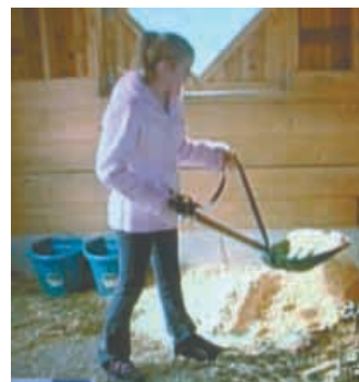
Shovel strap lets you shovel without bending over. It's held in place by two U-bolts.
