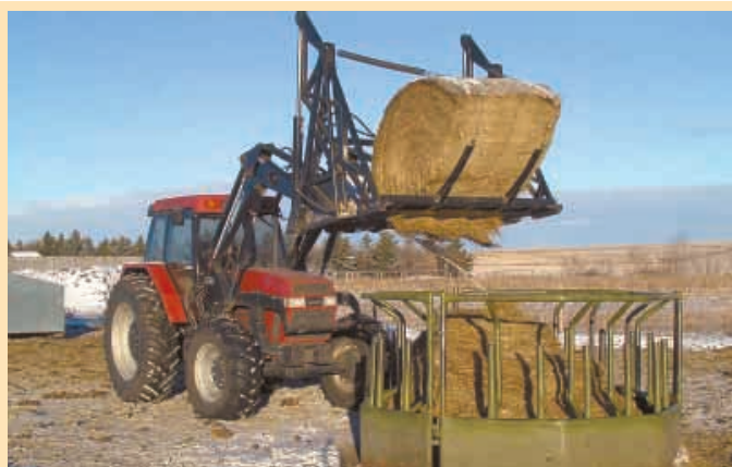
When jaws close, lower half of bale falls away and upper half is held in the bale cutter.
