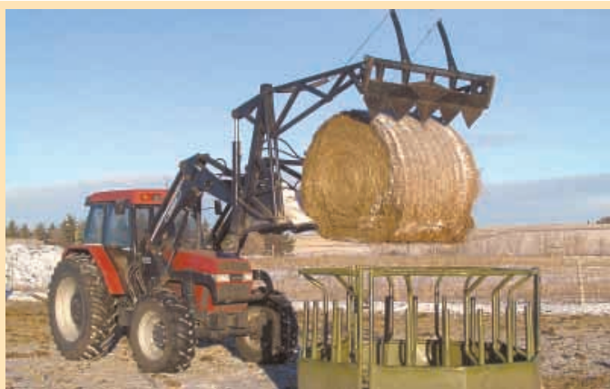
Bale cutter has a hydraulically-operated upper jaw with five large, sharpened cutting teeth that slice through bale.
