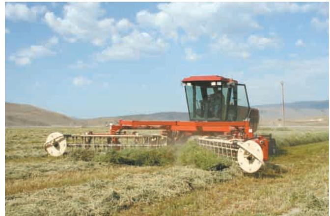
You can use the Bootsma front-mounted hay rake on an older swather, or on a new one. The mounted twin rakes simply mount in place of the header.
