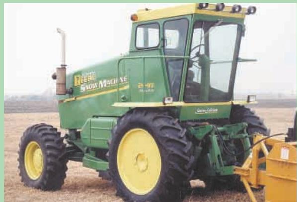
The pto-driven snowblower mounts on a 3-pt. hitch that bolts onto combine's front axle. Blower spout operates hydraulically from inside the cab.
