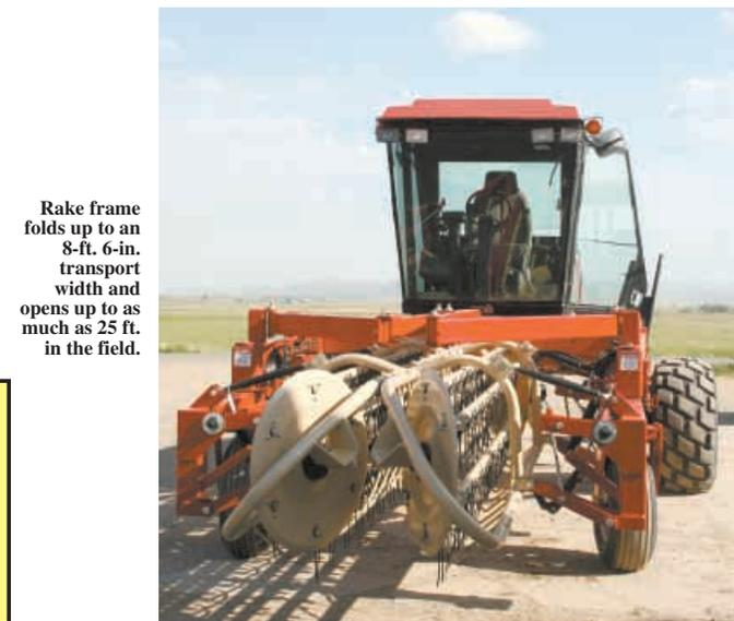
Rake frame folds up to an 8-ft. 6-in. transport width and opens up to as much as 25 ft. in the field.
