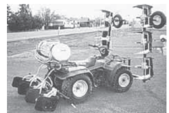
Three-piece bar has fold-up wings that mount on front of ATV. Boom on back covers the center rows.
