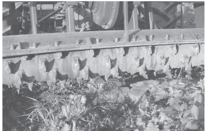
Stump grinder is equipped with carbide-tipped teeth.
