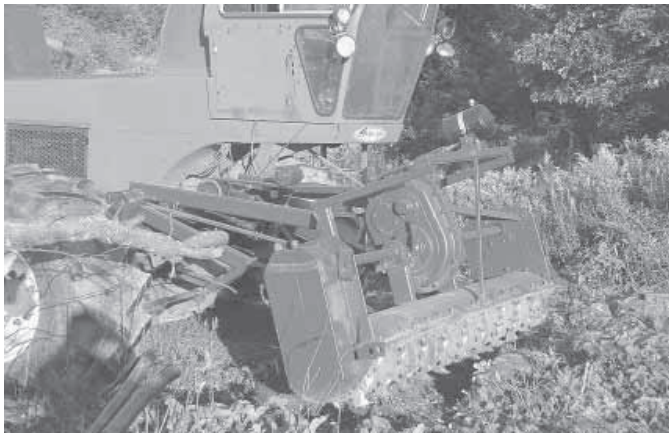
Ashton mounted a stump grinder on front of a New Idea Uni Harvester power unit.
