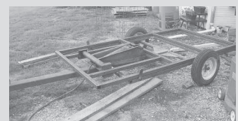
Hoist cylinder and scissors assembly mounts between two frames.
