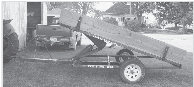
Mike Hoy built his own hydraulic dump trailer out of a 5 by 8-ft. trailer frame.
