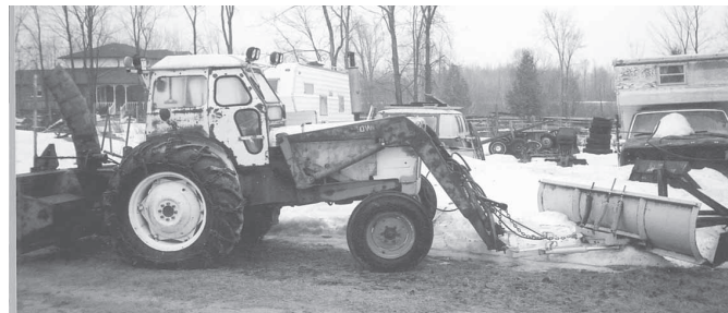
Ron Gardner uses a 6 1/2-ft. wide snowblower on back of his tractor and a 7-ft. wide truck snowplow blade on front.
