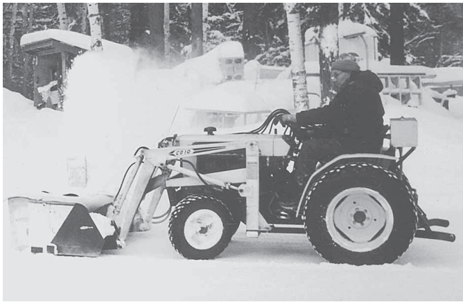
By mounting a snowblower in his loader bucket, Wolfe Lundgren can easily control its working depth, and even lift blower high enough to remove a bank of snow.
