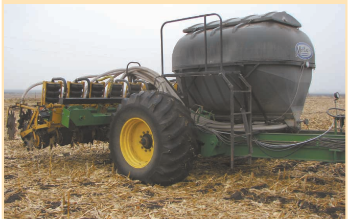
A 6-ton dry fertilizer tank from Montag Mfg. mounts on cart frame. Tank's fan-powered distribution system blows fertilizer behind deep till coulters on row units.
