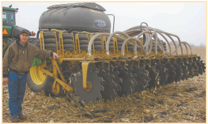
Mike Hermanson says his 12-row strip-till machine produces beautiful 10-in. deep by 10-in. wide zones, and also applies fertilizer in a single pass.
