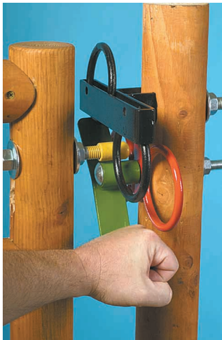
When lever is pressed down (left), one ring is lifted out of the way. When lever is released, gate begins to open.
