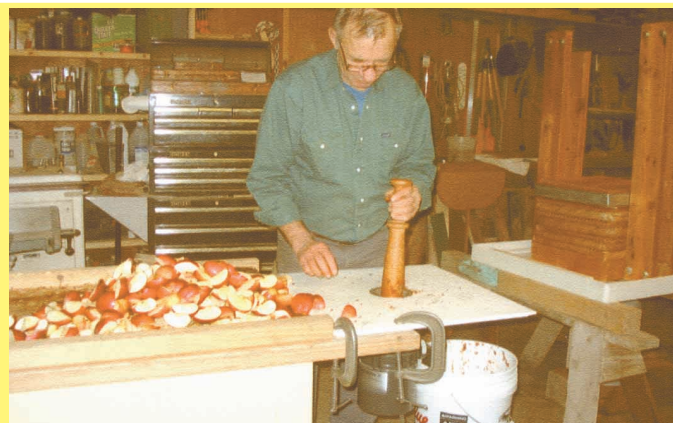
Chandler's first step to making great cider is to run it through a garbage disposal set up specifically for that purpose. It mounts on the underside of a sheet of plywood.
