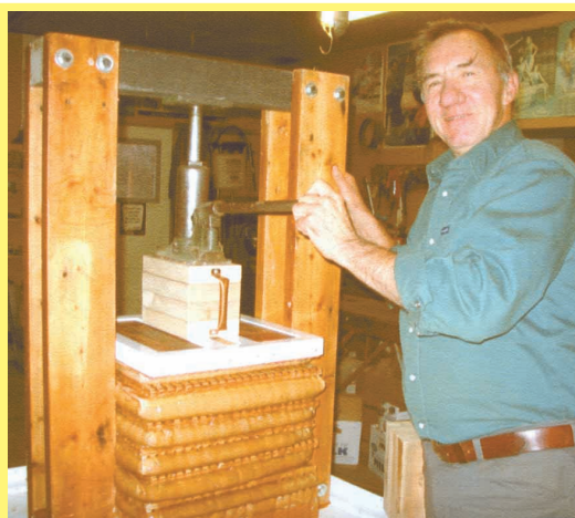
Hydraulic jack-powered press is used to squeeze out the juice from apples. The press sits in a plastic shower base that acts as a catch basin.
