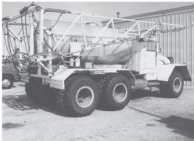
"I'm really happy with how it turned out," says Bob Greenwood, who turned a 2 1/2-ton Army 6-WD truck into a self-propelled sprayer.
