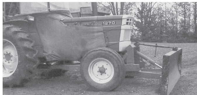
"It works better than a loader for leveling dirt and pushing manure and snow," says Glen Woodside, who mounted a 7-ft. dozer blade on front of his White 1270 tractor.
