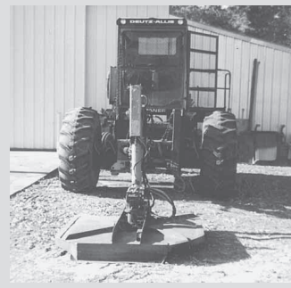
When arm is fully extended, the cutter head is a full 20 ft. from edge of combine.
