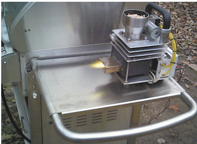
The "Pelletizer" is gravity fed, with no auger assembly and no bulky blower.
