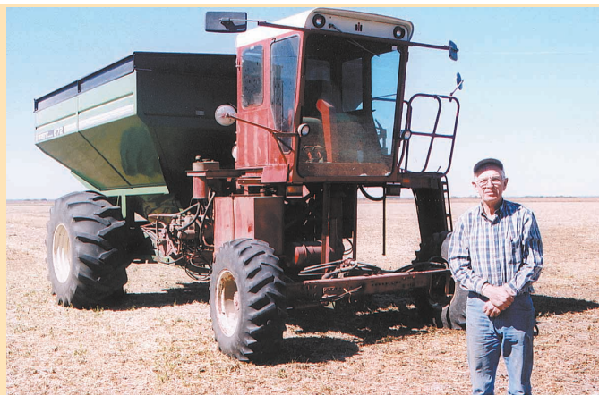
Noel Hicks and the self-propelled grain cart he built out of an IH 1480 combine.
