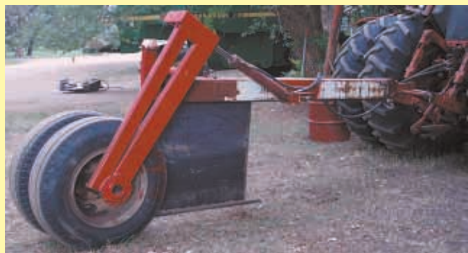
Home-built trenching plow buries wire down to 36 in. deep. Wire feeds through a tube located just behind plow blade.
