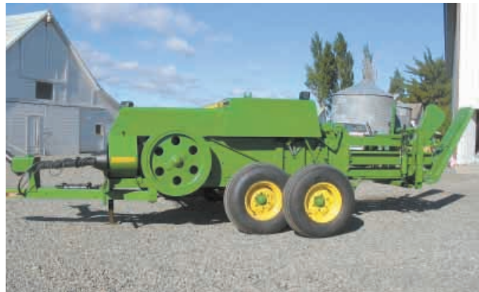
“Green Baler” is a heavy duty remake of the old Deere 468, with some improvements.
