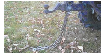
A pair of ground chains attach to ATV’s rear hitch to complete the circuit.
