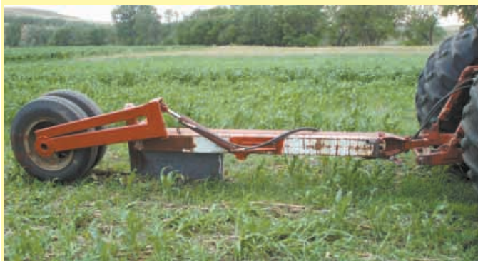
Skretteberg’s 3-pt. mounted trenching plow was built using the beam from an old row crop cultivator and the dual wheels off a flatbed trailer.
