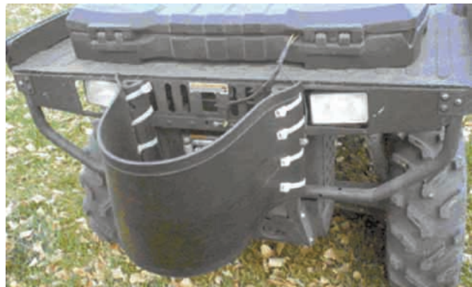
U-shaped rubber bumper conducts electricity. It extends 20 in. in front of ATV.
