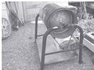
An old metal bed frame was cut down to make two A-frame supports for the tank.
