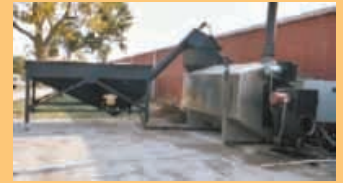
Furnace has the ability to burn high moisture biomass - up to 75 percent. Rocks, dirt or other contaminants do not affect operation.
