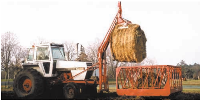
High-reach stacker can also turn bales sideways, if needed.
