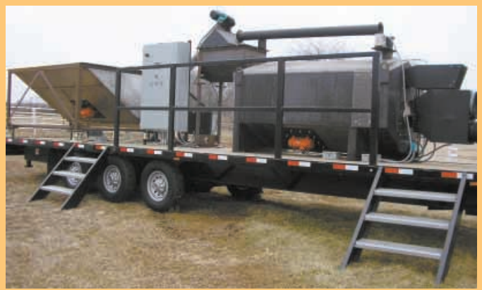
Furnace is shown here mounted on a trailer as a demonstrator unit.
