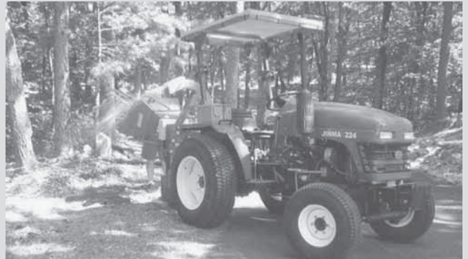
Completed tractor has a 3-pt. hitch, pto and a front weight rack. Shelley says it runs great and has only had a couple small problems in four years of use.
