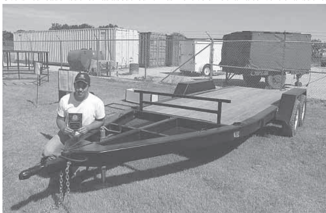
Jordan Dettmer, a high school senior, used Hesston swather tongues to build this heavy duty, 30-ft. long flatbed trailer.
