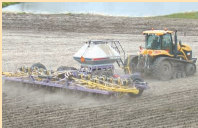
Mark Bauer's custom built 16-row Soil Warrior combines fall and spring tillage into one machine, including dry fertilizer application.
