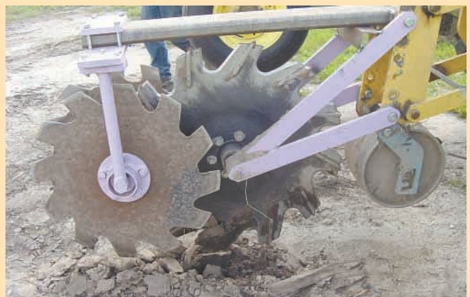
A massive 34-in. dia. primary coulters on each row unit has 5-in. long ductile iron bits. Two 26-in. following coulters fold soil into a neat berm.
