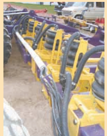
Air bags provide uniform down pressure to each row unit. The main toolbar serves as the air chamber, and pressure is regulated from 5 to 60 psi by a dial in the tractor cab.
