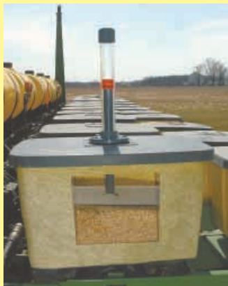
Seed level indicator installs on one or more of your planter seed boxes.
