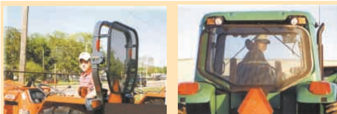
Expanded metal shield protects both driver and tractor from flying debris when mowing with a bush hog. Shield simply bolts to tractor's ROPS or to the back of cab.
