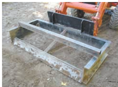
Blade with a 45 degree cutting edge mounts on front of land plane, eliminating the need to first tilt the device like you would a standard bucket.
