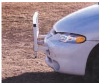
He used 1 1/2-in. sq. tubing for the 72-in. wide guard.
