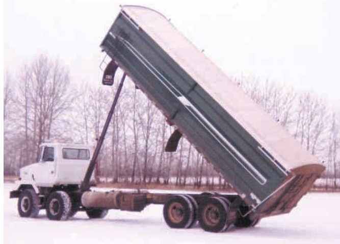
Beamish mounted a 28-ft. long grain box on this 1990 Autocar truck equipped with twin steering axles. Box is fitted with a 45-ton, 5-staged telescopic hoist.
