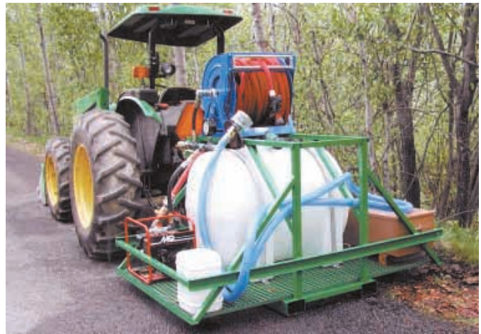
Self-contained fire fighting rig includes a 225-gal. water tank with Hypro pump, 100 ft. of fire hose and storage compartment for tools.
