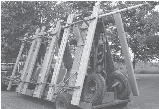
Two 11-ft. uprights spaced 19 ft. apart support a 29-ft. long horizontal bar which the picnic tables lean against. Carrier can haul six 10-ft. tables at once.
