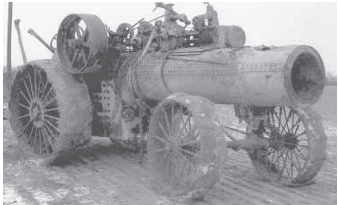
Once it was out of the muck, a fire engine sprayed 2,500 gal. of water on the old steam engine to clean it off. The tractor was being used to build a bridge over the Republican River when it got pushed into the river during a flood in 1935.
