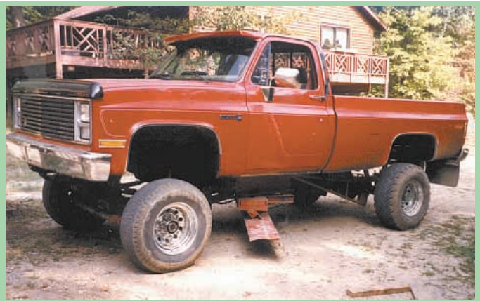
Home-built, articulated "belly blade" can be automatically angled from side to side, and also tipped up and down to change the angle at which it enters the ground.
