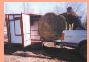
Double doors on one side of feeder swing out for easy loading.
