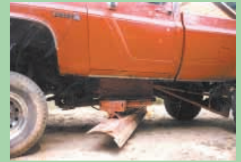
To provide maximum support, blade is secured to plate it's mounted on at five different places.
